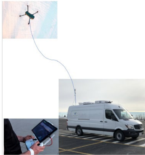
Figure 2. Real time measurements of benzene and VOC at different altitudes using a UAV with the PTR-TOF-MS mobile platform.
