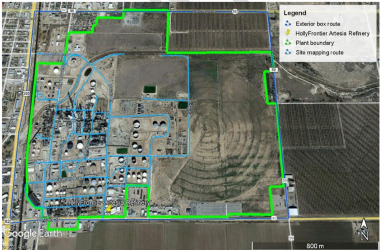
Figure 5. The facility map and the routes in which the measurements will be conducted. The cyan line indicates the locations in which ground level measurements will be conducted using the mobile lab. The blue line indicates the route in which downwind fenceline measurements will be conducted at the ground level and at high altitude measurements using the mobile lab and the UAV. The green line is the plant boundary.
