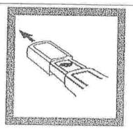
5. Remove the instrument cap.
