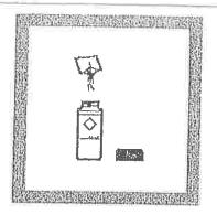
2. Add the contents of one DPD Total Chlorine Powder Pillow to the sample cell (the prepared sample). Cap and gently shake for 20 seconds.
