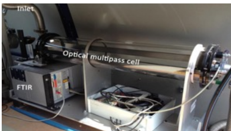
Figure 3 The MeFTIR instrumentation consisting of a Bruker FTIR spectrometer connected to an optical multi-pass cell.
