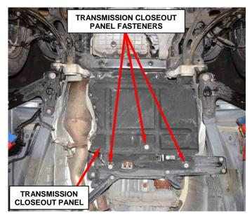
**Figure 2 – Transmission Closeout Panel**
