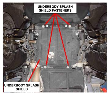
**Figure 1 – Engine Closeout Panel**
