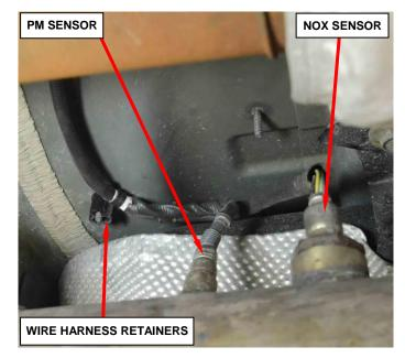
**Figure 11 – Wire Harness Retainers**
