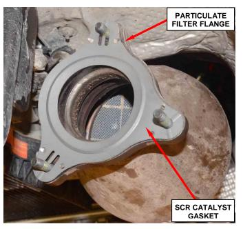
Figure 18 – SCR Catalyst Gasket
