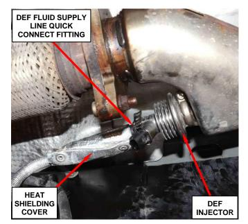
**Figure 22 – DEF Injector Fitting**
