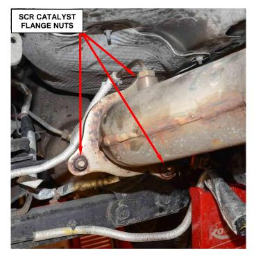
Figure 30 – SCR Catalyst Flange
