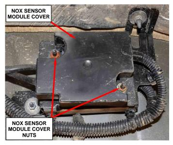
Figure 8 – NOx Sensor Module Cover
