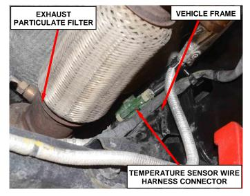
Figure 20 – Exhaust Temperature Sensor
