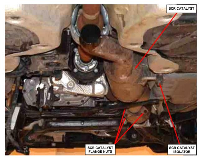
Figure 14 – SCR Catalyst Assembly
