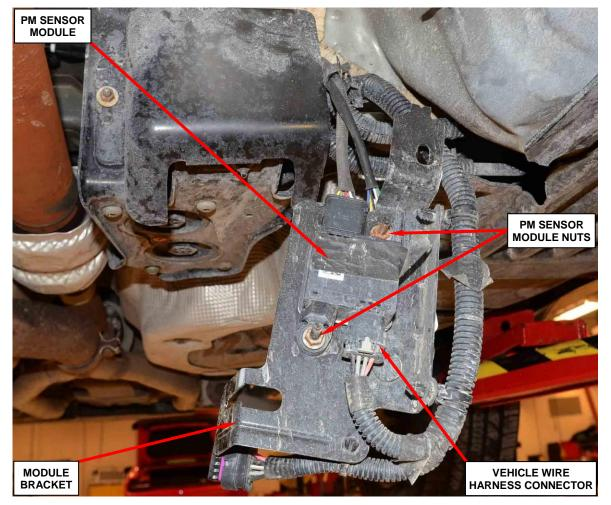
Figure 10 – PM Sensor Module
