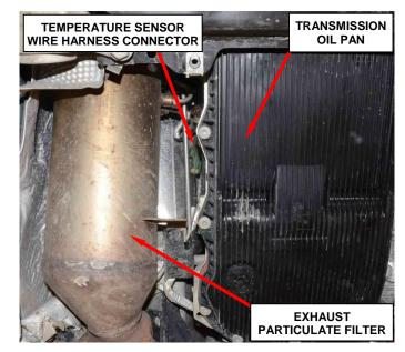
**Figure 4 – Exhaust Temperature Sensor**
