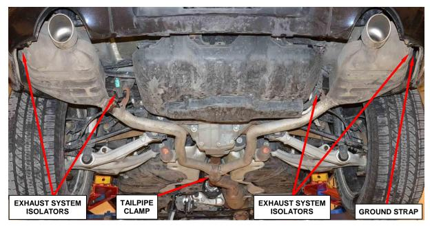
**Figure 13 – Tailpipe and Resonator Assembly**
