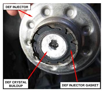
Figure 17 – DEF Injector Gasket
