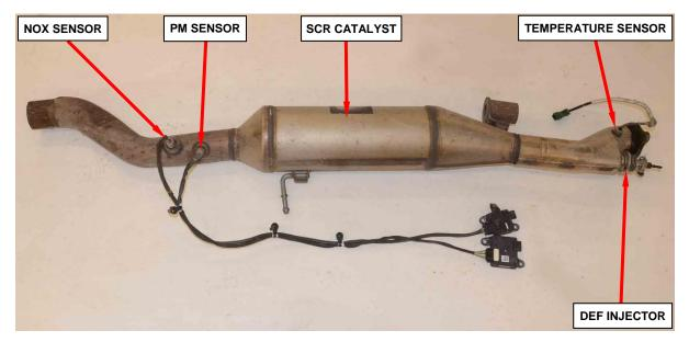
Figure 15 – Selective Catalytic Reduction (SCR) Catalyst Assembly
