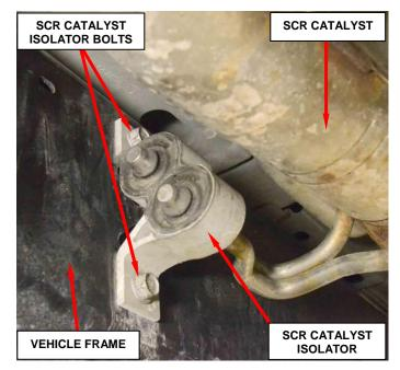
Figure 29 – SCR Catalyst Isolator
