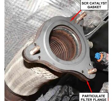
Figure 35 – SCR Catalyst Gasket
