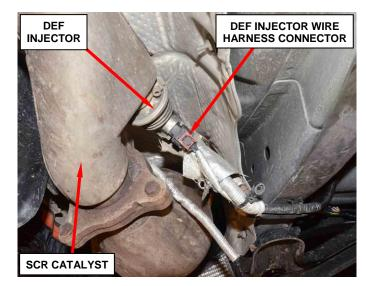
**Figure 5 – DEF Injector Harness**
