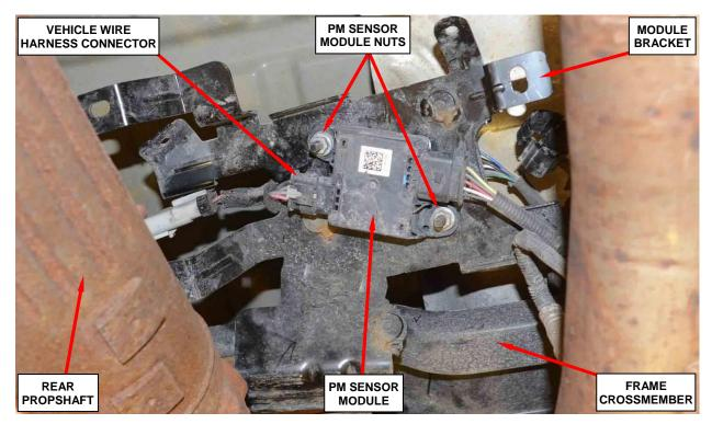
Figure 25 – PM Sensor Module
