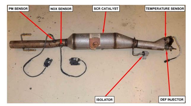
25. Transfer the isolator to the **NEW** SCR catalyst (Figure 32).
