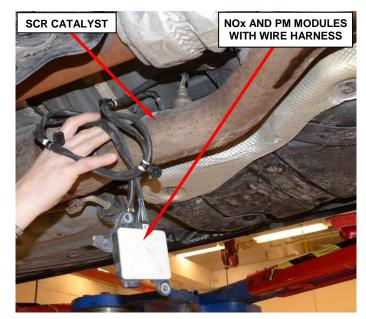
**Figure 12 – Wire Harness with Modules**
