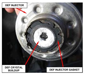
Figure 34 – DEF Injector Gasket
