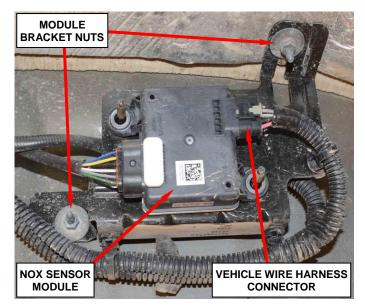
Figure 9 – NOx Sensor Module
