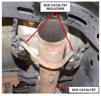
**Figure 31 – SCR Catalyst Isolators**
