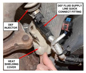
**Figure 6 – DEF Injector Fitting**
