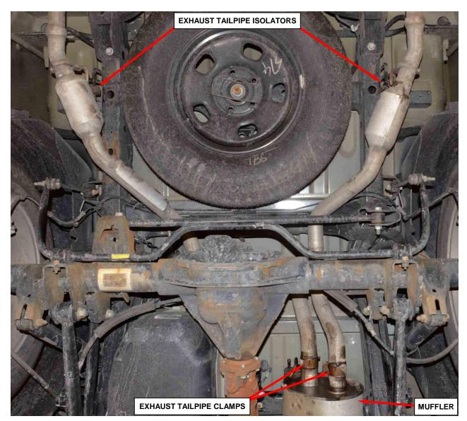
Figure 27 – Tailpipes (Dual Exhaust Shown Single Exhaust Similar)
