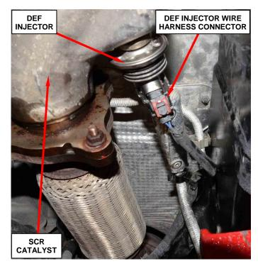
**Figure 21 – DEF Injector Harness**
